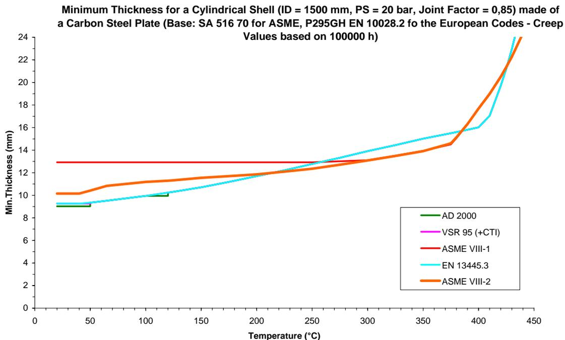
In the graph, which shows the minimum required thickness of a cylindrical shell at different temperatures using different pressure vessel codes). It has also to be noted that **the new Division 2 can now be used also in the creep range** (the creep values are the same of Division 1).
